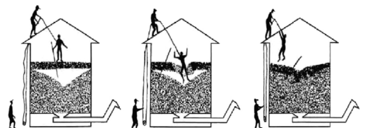
Figure 3. Accumulation on bin side that results in engulfment.
